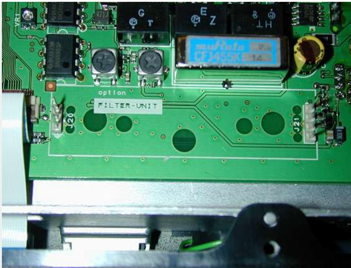
3. Here's the filter correctly oriented ready to be put in. Note that the 3 pin connector is on the LHS and the 4 pin connector on the RHS. The filter is installed writing side up as shown.
