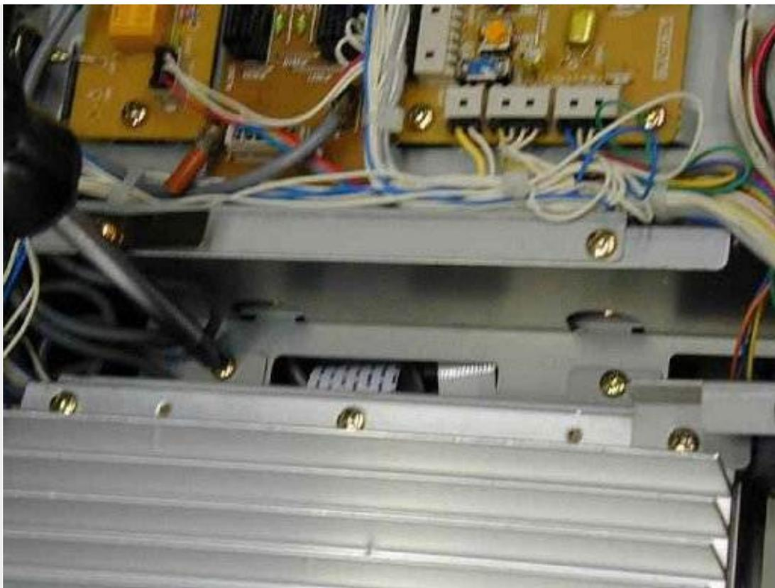
Four main screws hold the heatsink mounting bracket. Two screws are shown above (one under the screwdriver and one a few inches to the right of it). Two more screws are on the side of the radio chassis. You might want to remove the long screws holding the fan bracket, although I got by without doing so.
