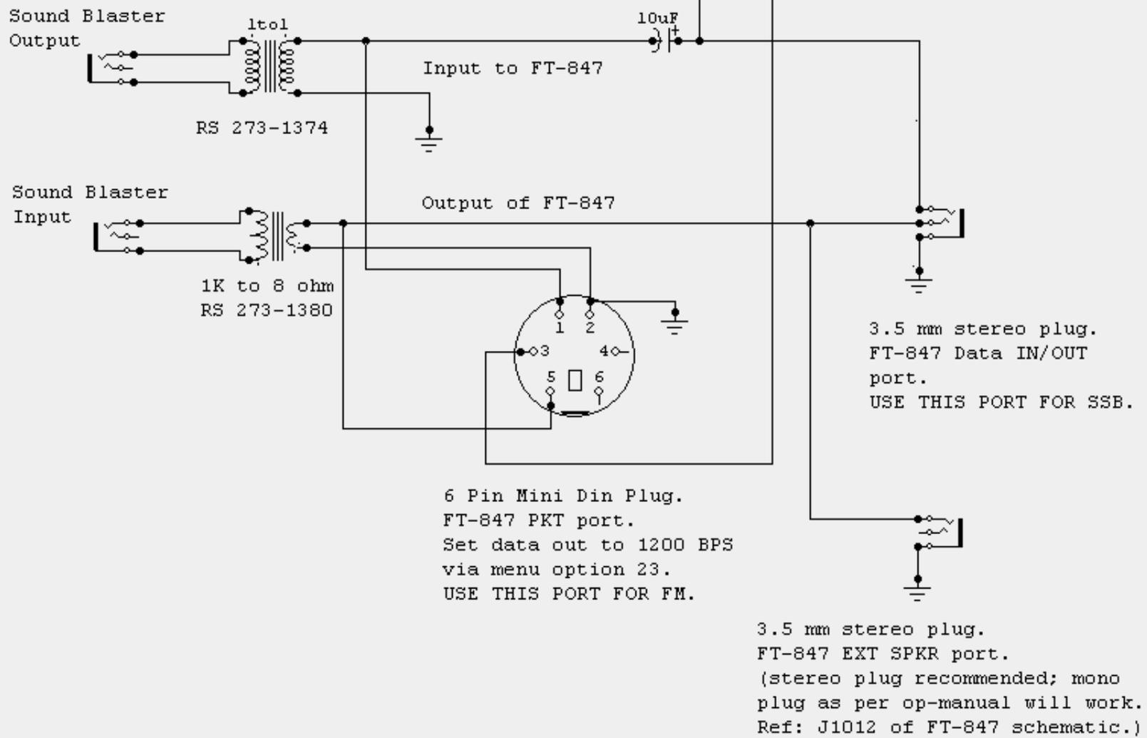
**Note.** Due to the low voltage output levels of the PKT and Data IN/OUT ports, it is recommended to use the EXT SPKR port as output to the sound blaster. This will ensure proper SSTV signal triggering and synchronization.
