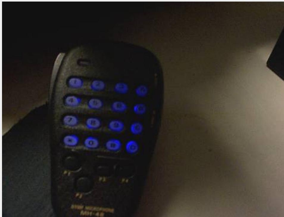
I ordered LED's from Newark Electronics [www.newark.com](http://www.newark.com) and they came in two days with no problems. I ordered part # 98B5036 which are size 805 surface mount, blue, low-profile with a veiwing angle of 170 degrees. The higher the veiwing angle, the better the light will diffuse behind the buttons on the mic. These LED's are made by Agilent Technologies (part #HSMB-C170) and where about 65 cents a peice. They do have a minimum order of \$25.00 though but they are worth it.
