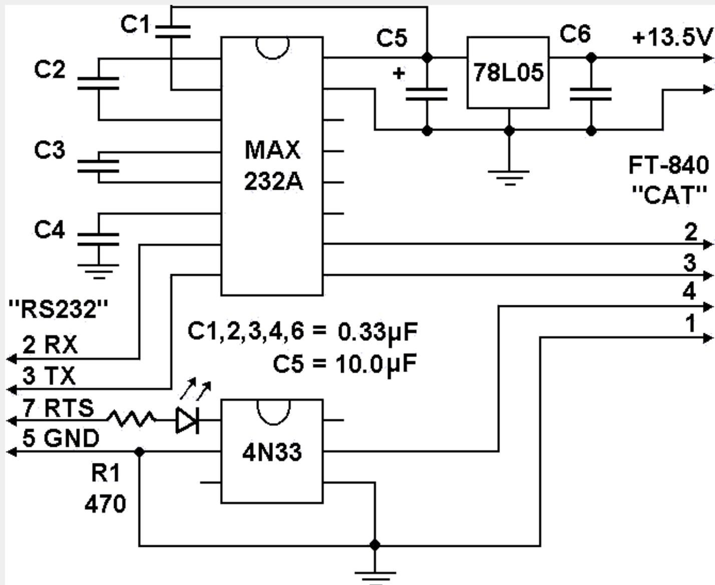
The heart of this interface is MAX232A. You can use any similar chip MAX203, MAX232, MAX233, but check documentation for proper connections. Power supply +5 volts is coming from voltage regulator 78L05 that takes +13.5 volts from the back of FT-840 radio (RCA connector). PTT controlled via optocoupler 4N33 by the RTS signal from RS-232. I used DB9 serial port. If you use DB25, then you have to change pin numbers according DB25 assignment. CAT plug is 6 pin Mini DIN.
