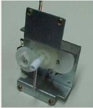
Photo 3: Mechanical indicator needle system
