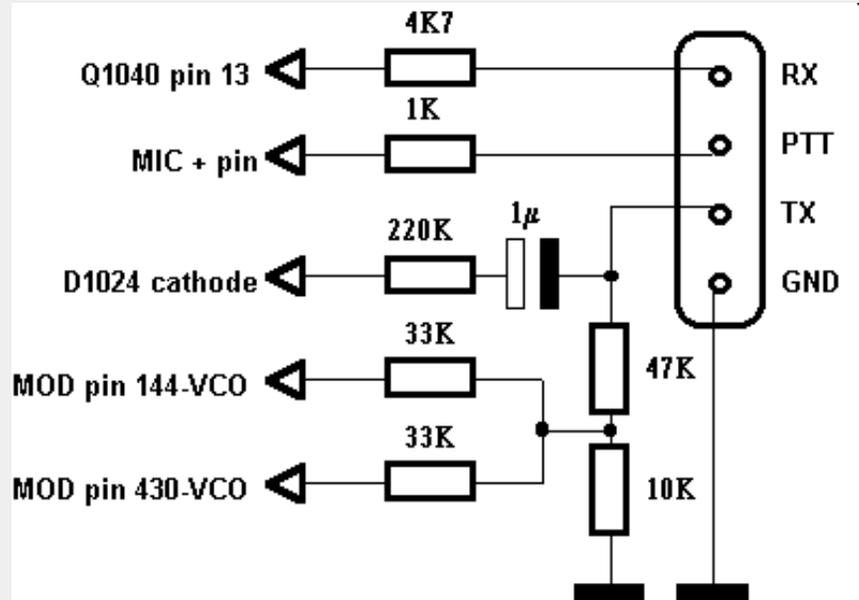
Due to existing varicap diode modulator we'll need only very few new parts. The correct values are found after modifying 4 set of FT-50 radios. Because of space restriction I suggest the use of a (47k/10k) resistive voltage divider and not even the smallest pot. You can increase the value of the 1µF capacitor to improve low-frequency response.
