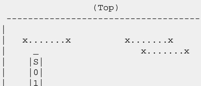
You have to solder the jumpers marked x....x, either by connecting the soldering points on the back, or inserting the jumpers through the holes on the front.
