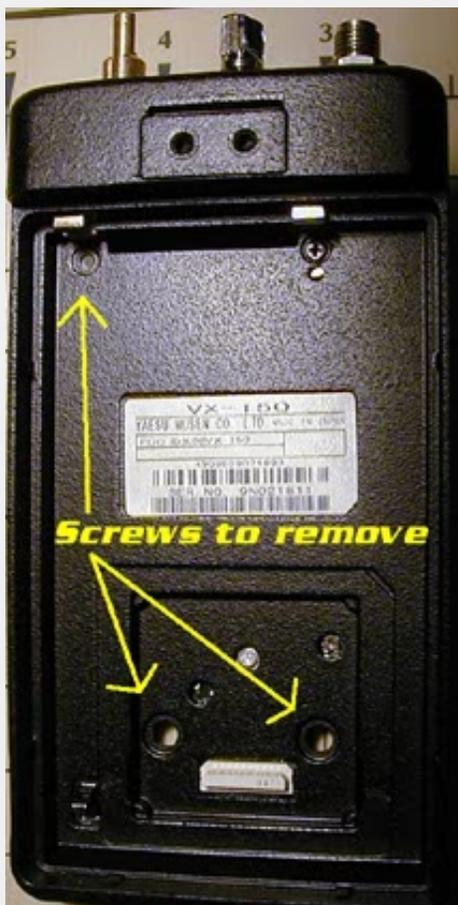
Fig 2 Remove screws
