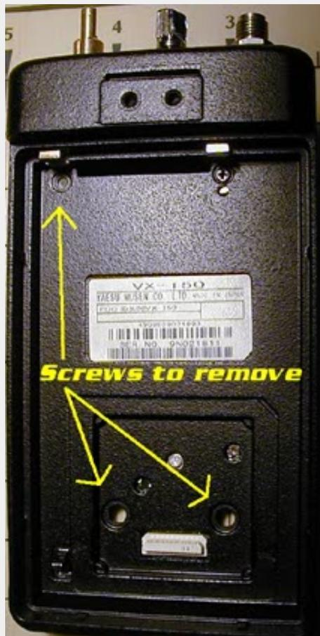
Fig 2 Remove screws
