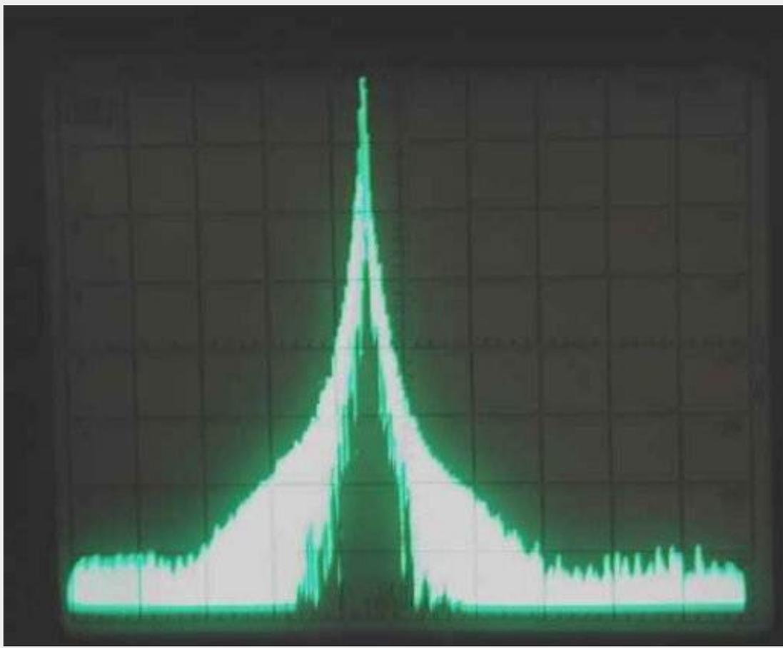
The 751A is approximately -58 dB at 1 kHz, and rolls off smoothly.
